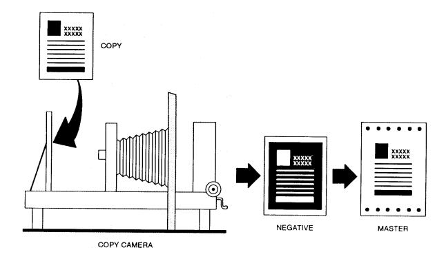
Figure 10-3. Offset photographic process.
