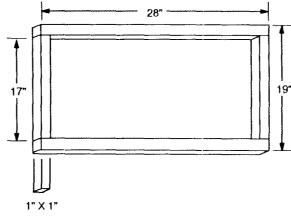
Figure F-4. Materials and measurements for constructing base and cover.
