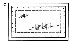
Place a row of tacks along the remaining edges of the frame. The fabric must be pulled tight before driving each of these tacks.
