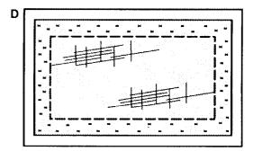
Continue to drive the tacks around the inside edge of the frame to give added strength to the screen.
