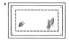
Place the fabic over the wooden frame and place one tack in each corner to hold the cloth in place. Use either small 1/4-inch tacks or staples. Approximately 90 tacks or staples are needed to attach the fabic securely.
